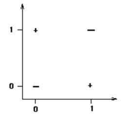
XOR is a function that cannot be learned by a perceptron: let + correspond to output 1 and – to output 0, then XOR is not linearly separable
